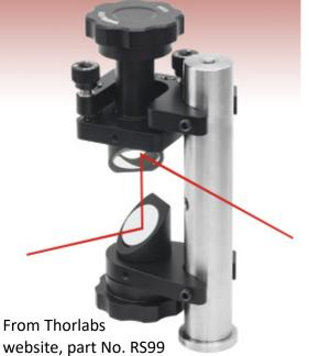
Periscopes are a location where extra caution is needed, since the beam is intentionally steered up/down from the table (i.e., where your eyes might be)
